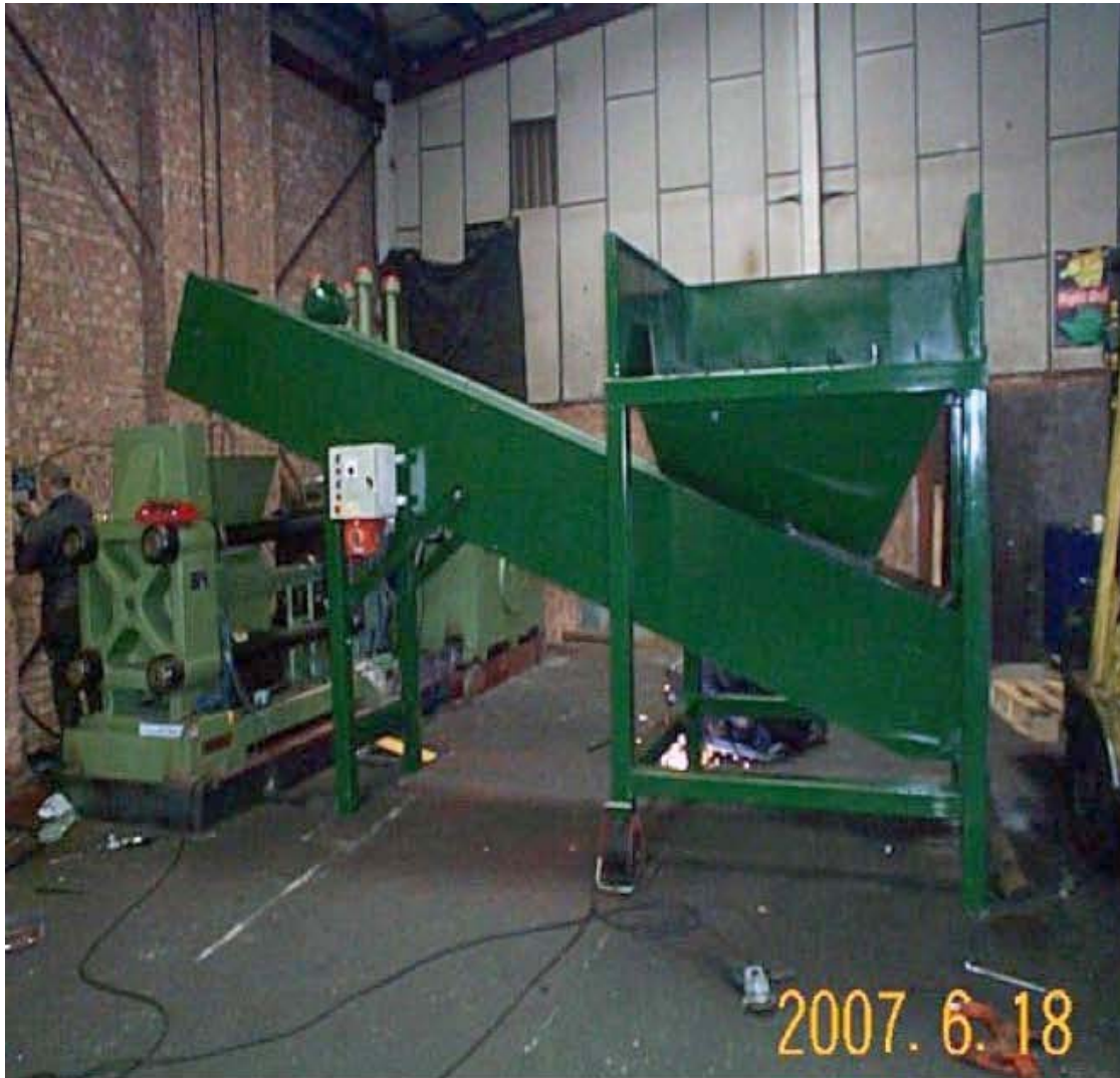
Briquetting press used in UK – Aluminum Briquetters
